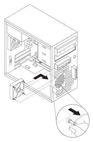
Figure 29. Installing the front fan assembly
